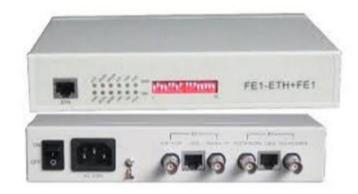
**PRODUCT OVERVIEW:** - AT-CSU-DSU is an 10/100M Ethernet and FE1 to E1 converter, provides two E1 interfaces and one FE interface. It can extract several consecutive timeslots from the up-E1 (N×64Kbps), to transmit Ethernet traffic. The left timeslots of the E1 are used to transmit E1 traffic between the up-E1 and down-E1. The Ethernet traffic and down-E1 traffic are physically isolated.
