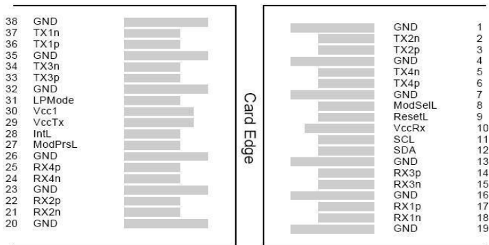
Top Side Viewed from Top Bottom Side Viewed from Bottom QSFP MSA-compliant 38-pin connector
